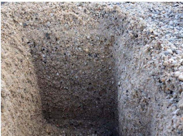
Figure 11 Small trial pit showing homogeneous sand build-up with a coarse top layer.
