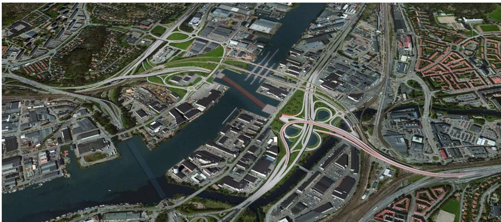
Fig. 2. Project overview (blue river crossing: Existing Tingstad tunnel; red river crossing: Marieholm tunnel) (source: Trafikverket).
