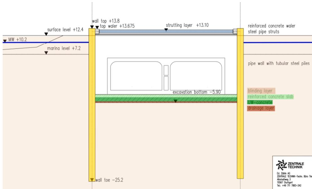
Fig. 7. Cross section of the construction pit (design section A-A).
