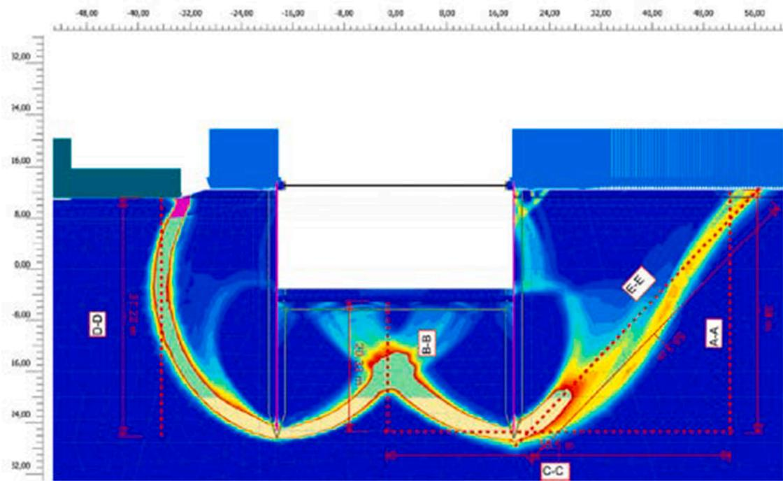
Fig. 11. Illustration of failure mechanism from a strength reduction analysis.
