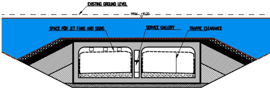
Fig. 3. Tunnel cross section.
