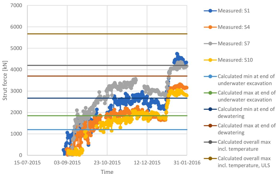
Fig. 12. Comparison between measured and calculated min (low water at + 9.6 m) and max (high water at + 12.3 m) strut forces. The struts are designed for “Calculated overall max including temperature, ULS”.
