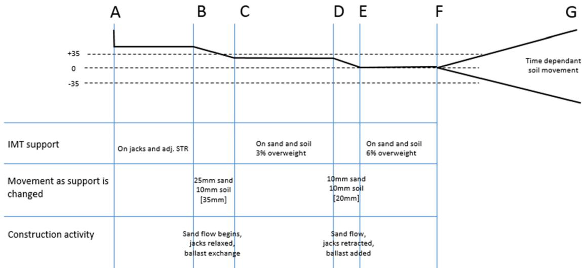
Fig. 23. Loading of tunnel and exchange of loads from temporary to permanent support conditions against initial settlement.
