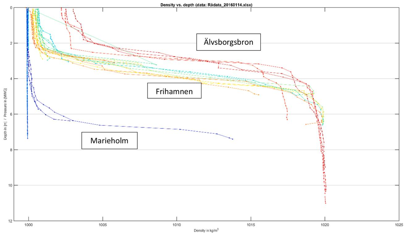
Fig. 16. Measurements of water density changes with depth measured at various moments (samples from Jan 14th 2018 at different times and locations at and downstream from the tunnel).
