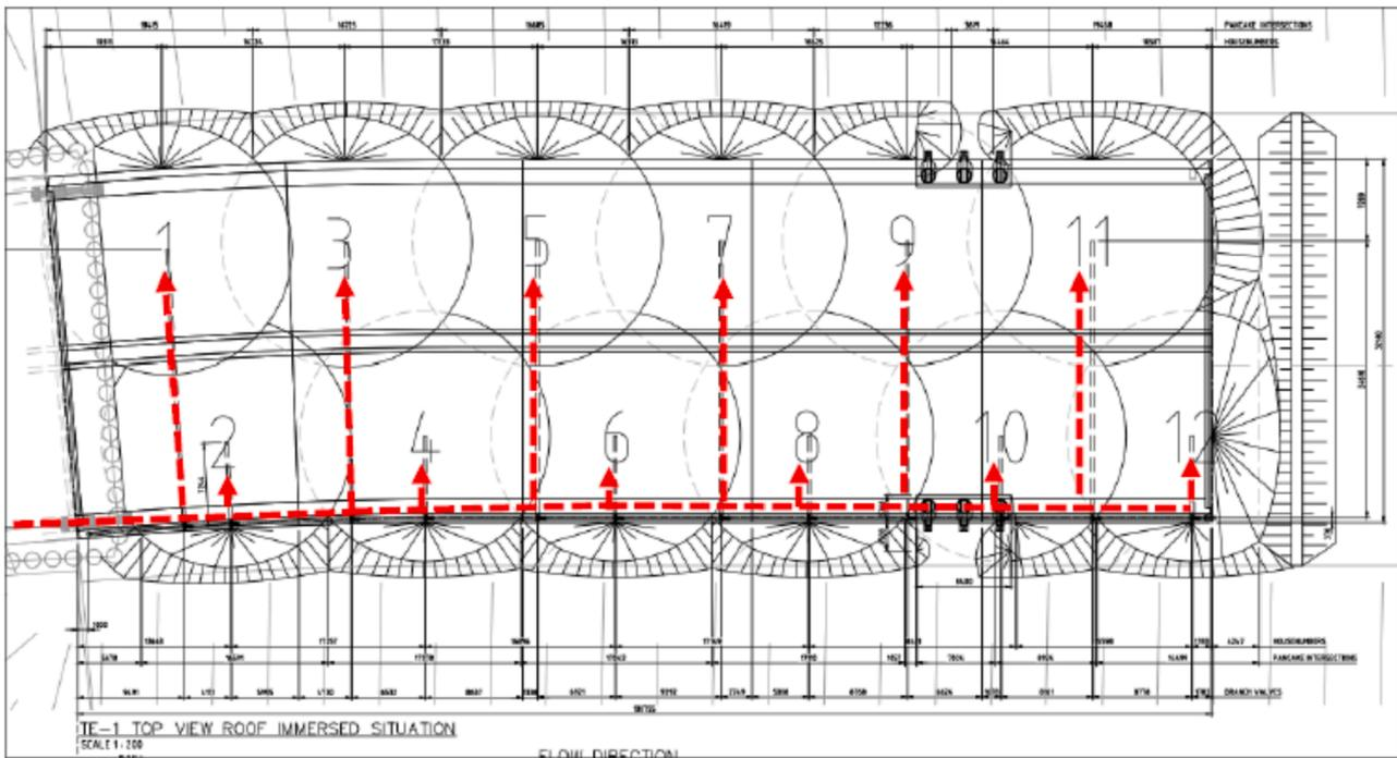
Fig. 22. Location of supply lines and sandflow “pancakes”
