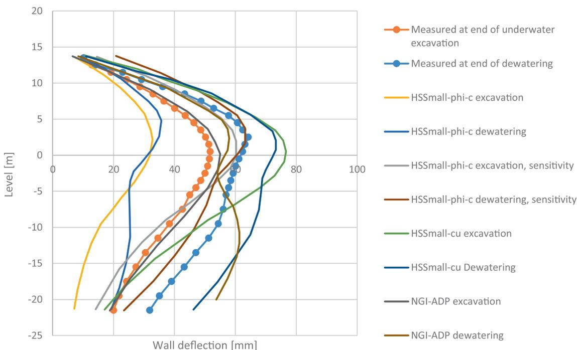
Fig. 9. Comparison between measured and predicted wall deflections (design section B-B, low water at + 9.6 m).
