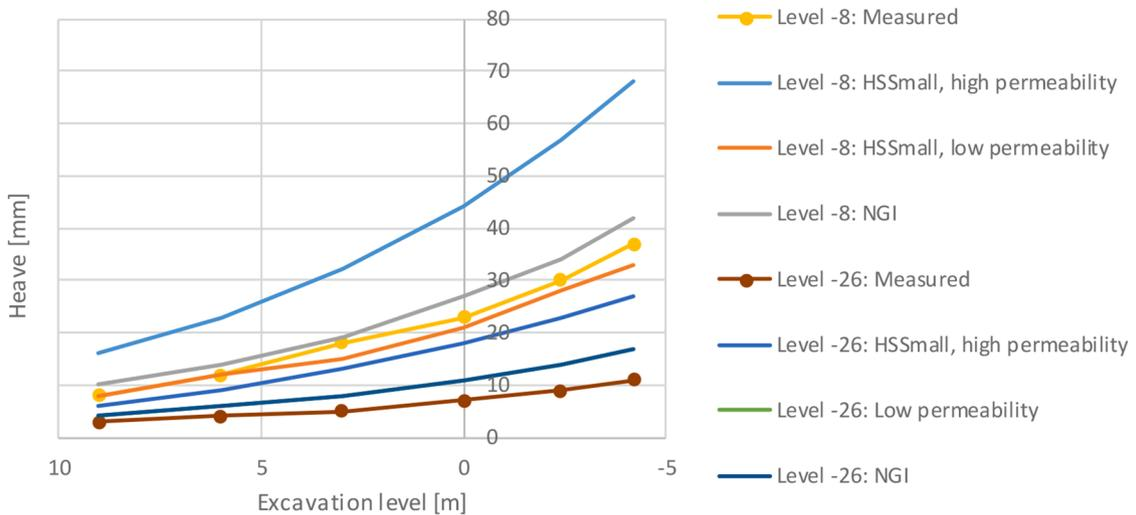
Fig. 10. Comparison between measured and calculated heave of the soil during underwater excavation.
