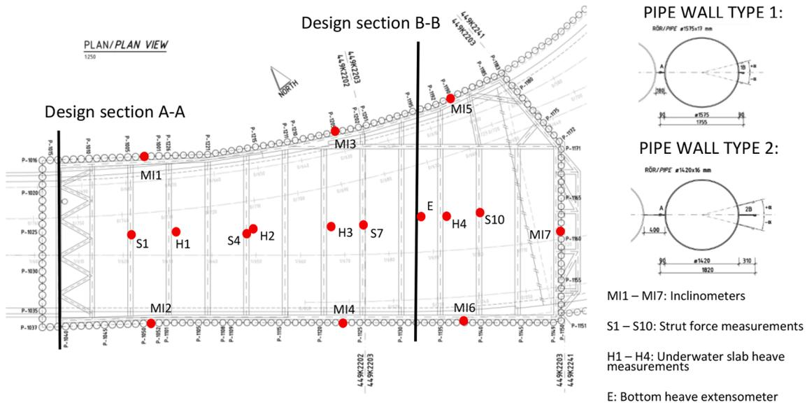
Fig. 6. Plan view of the construction pit.
