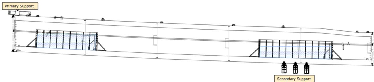
Fig. 19. Temporary support system for tunnel element 1 and 2.
