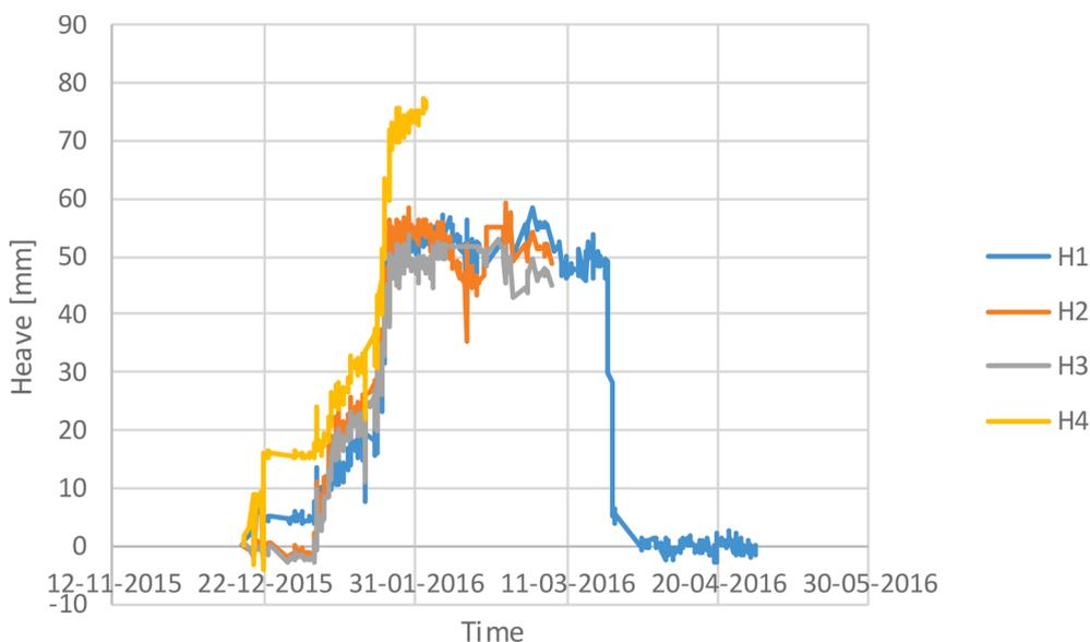
Fig. 13. Measured heave of the underwater slab.
