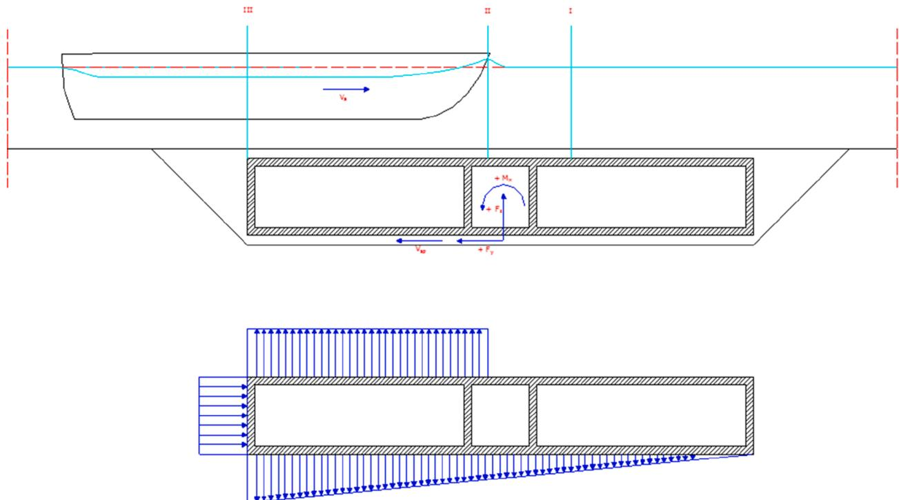
Fig. 18. Effects on tunnel element.
