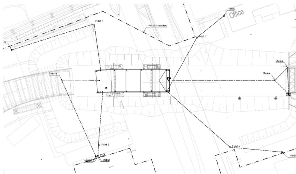
Fig. 17. Warping configuration for pontoon and tunnel element.
