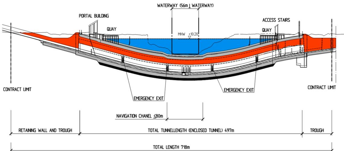
Fig. 4. Tunnel longitudinal section.
