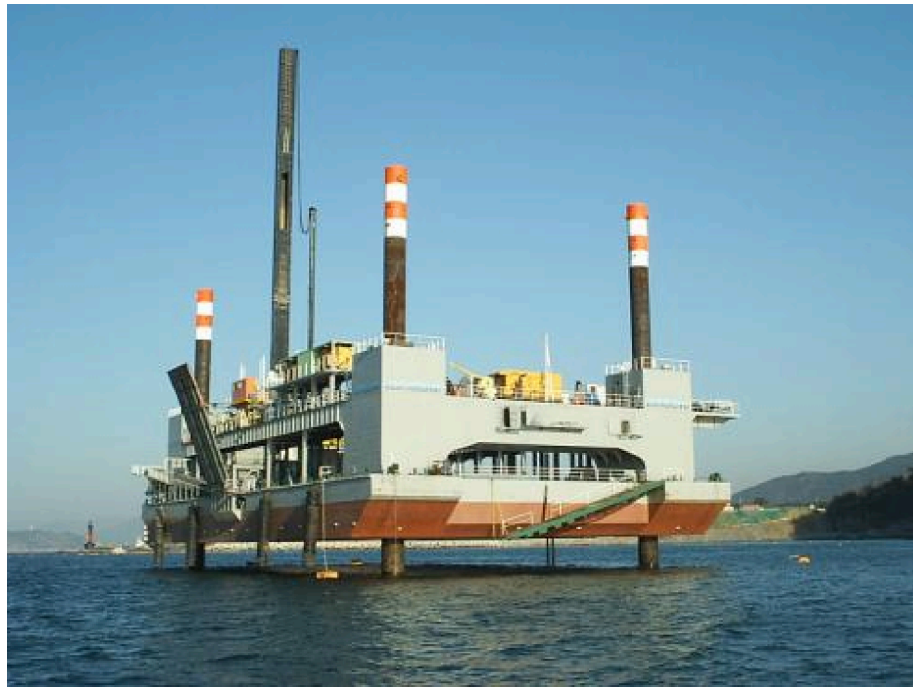
Fig. 8. Gravel bed placement barge KUS-ISLAND from Eunsung O&C.
